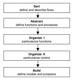
Fig. 3. Design steps for a distributed structure
