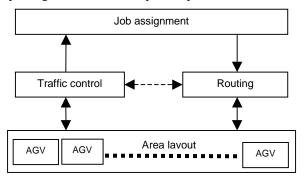
Fig. 6. AGV system with control functions.
