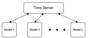
Fig. 4. Timer Server for synchronization
